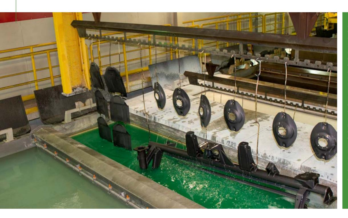
Cataphoretic painting (E-COAT) is used to cover elements that require coatings with significant corrosion resistance. At SaMASZ this process is carried out in a fully automated method. Each step is continuously monitored and archived, ensuring the repeatability of the process and the highest coating quality. In addition, it provides high weather resistance, corrosion protection, chemical and mechanical protection and an eye-catching design.
